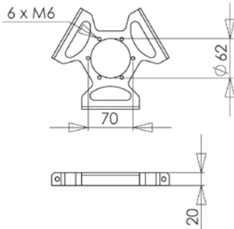
The design of the gripper that is mounted under the robot have great influence on the performance of the robot. Both the weight of the gripper and the distance of the center of gravity of the gripper to the TCP base point have negative influence on the final performance of the robot.
