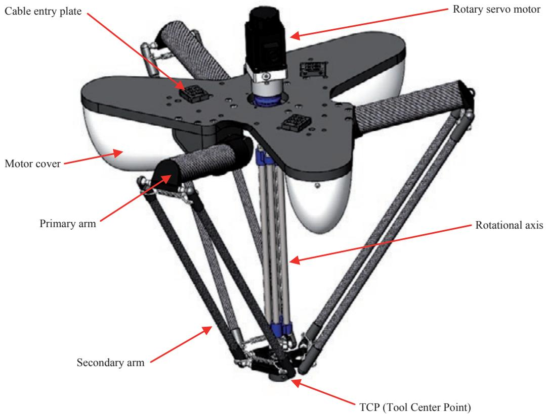
The CR\_UGD4\_XXL1300H robot consists of three radially placed axis which give the TCP freedom to move in three directions, X, Y and Z. An optional fourth axis can take care of the rotation, Rz, of the TCP.
